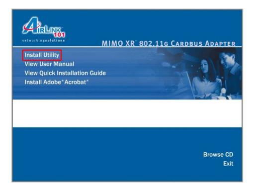
**Note:** If the Autorun screen doesn't appear automatically go to **Start**, **Run**, and type **D:\autorun.exe** (where **D** is the letter of your CD drive) and click **OK**.
