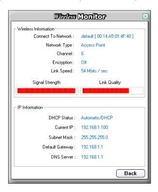
If you do not have adequate Signal Strength, try re-orienting the Access Point and/or the Cardbus Adapter to get a better reception.
