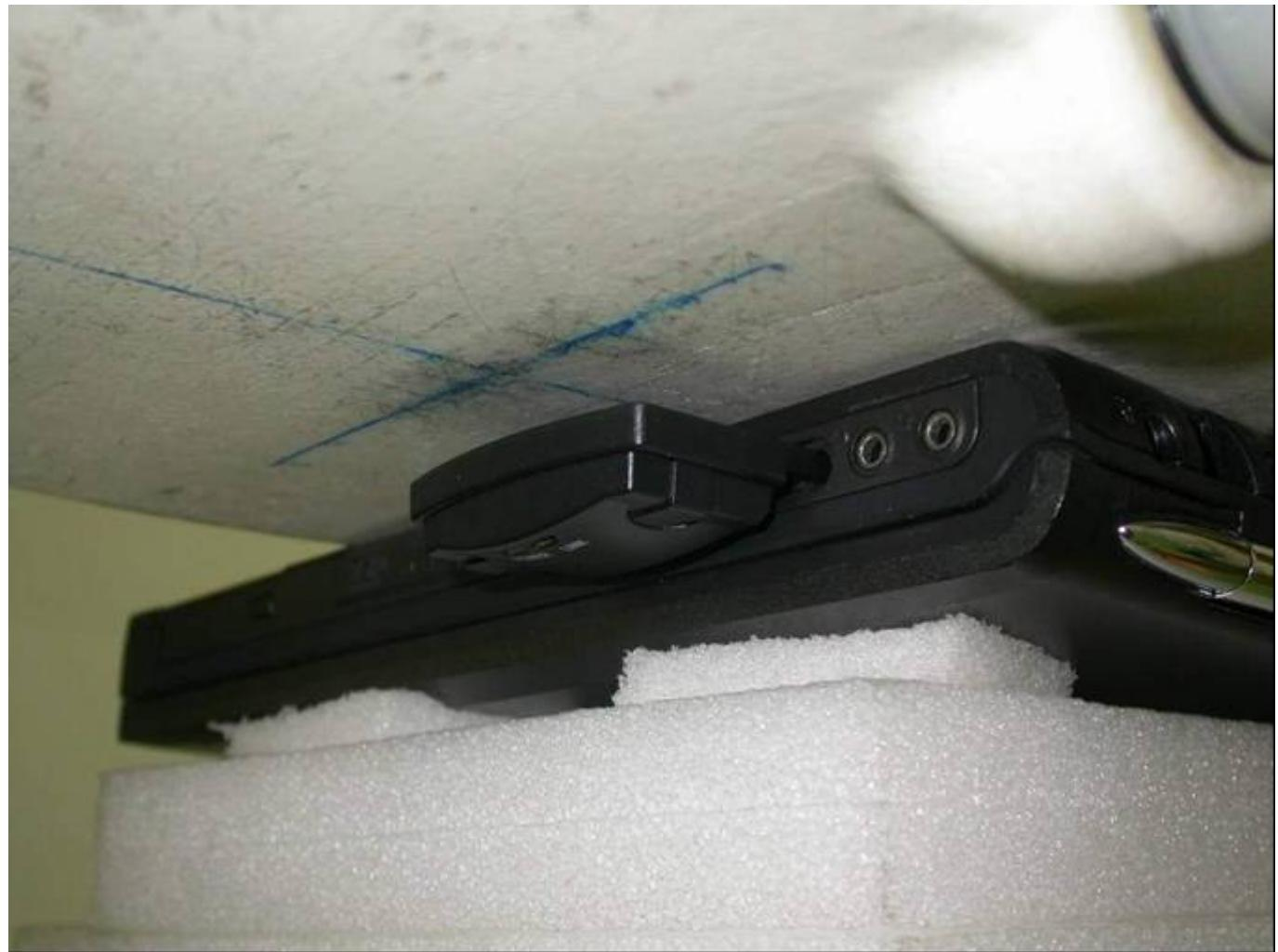
**The Bottom of the EUT to the flat phantom distance 12 mm**
