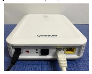
5. Plug other end of Ethernet cable into the Lumen support connections (ONT) or wall jack.
