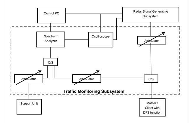
The test transmission will always be from the Master Device to the Client Device. While the Client device is set up to associate with the Master device and play the MPEG file (6 y Magic Hours) from Master device, the designated MPEG test file and instructions are located at: <a href="http://ntiacsd.ntia.doc.gov/dfs/">http://ntiacsd.ntia.doc.gov/dfs/</a>.
