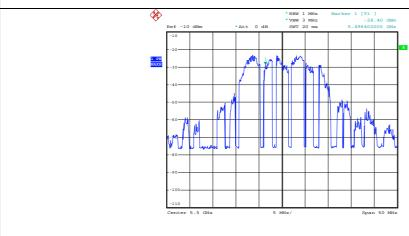
The client and DFS-certified master device are associated, and the movie can be streamed as specified in the DFS Order for a non-occupancy period test.
