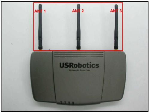
**NOTE:** When the EUT operating in 802.11b/g, the ANT 3 was the worst case and chosen for final test
