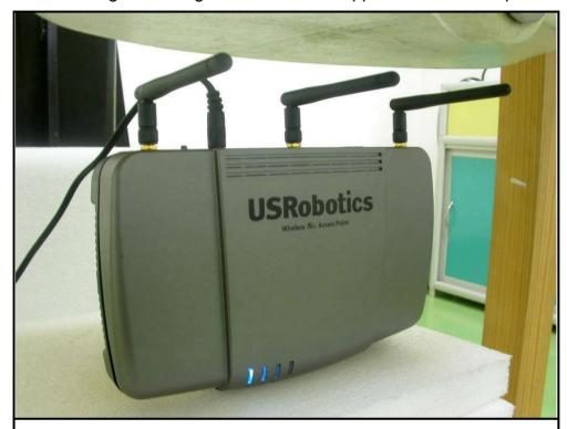
The bottom of the EUT face to the phantom with 15 mm-separation distance.
