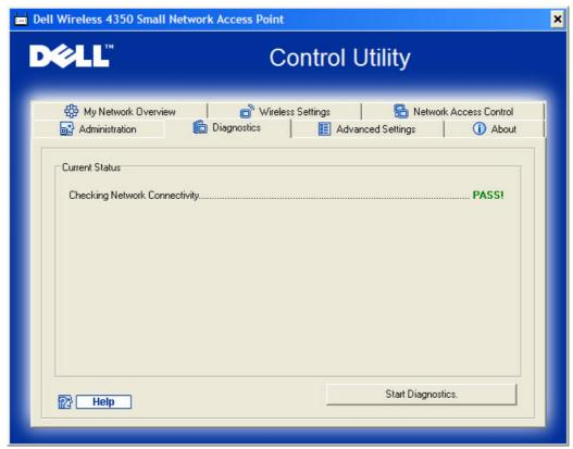
You can monitor the current status of your network connection in the **Diagnostics** menu. The network diagnostics can be activated by clicking the **Start Diagnostics** button on the bottom of the screen.
