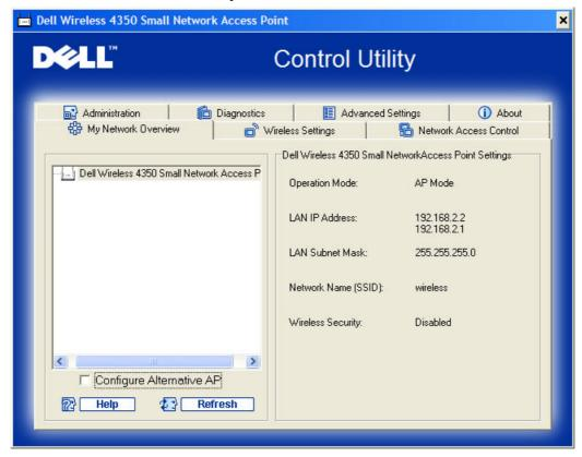
The Control Utility allows the user to manage multiple Dell Wireless 4350 Small Network Access Points on the network by allowing the user to configure an alternative access point to the default access point presented by the Control Utility.
