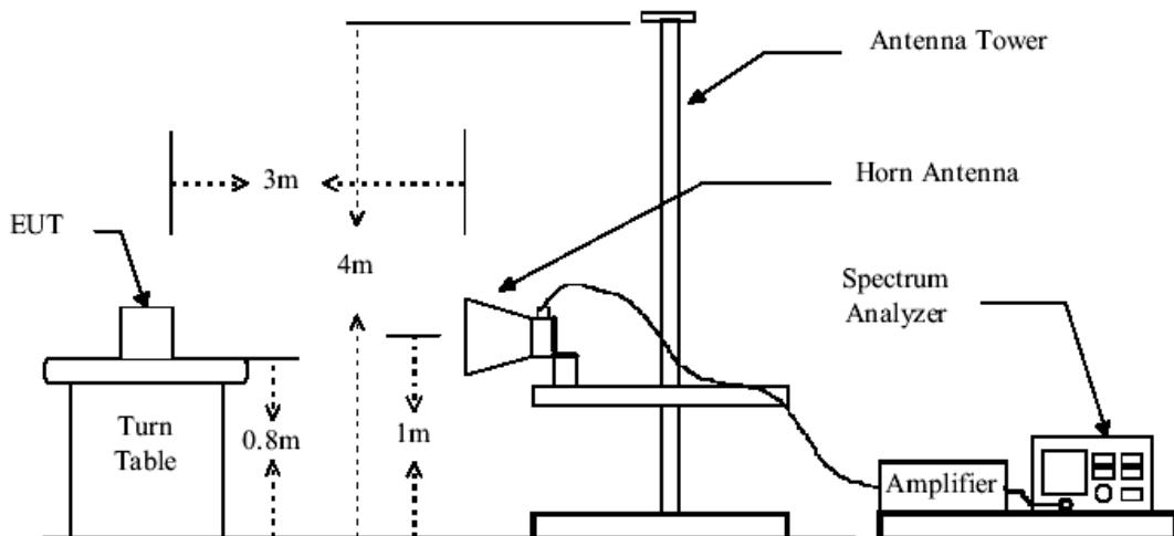
The field strength is calculated by adding the Antenna Factor, Cable Factor & Preamplifier. The basic equation with a sample calculation is as follows:
