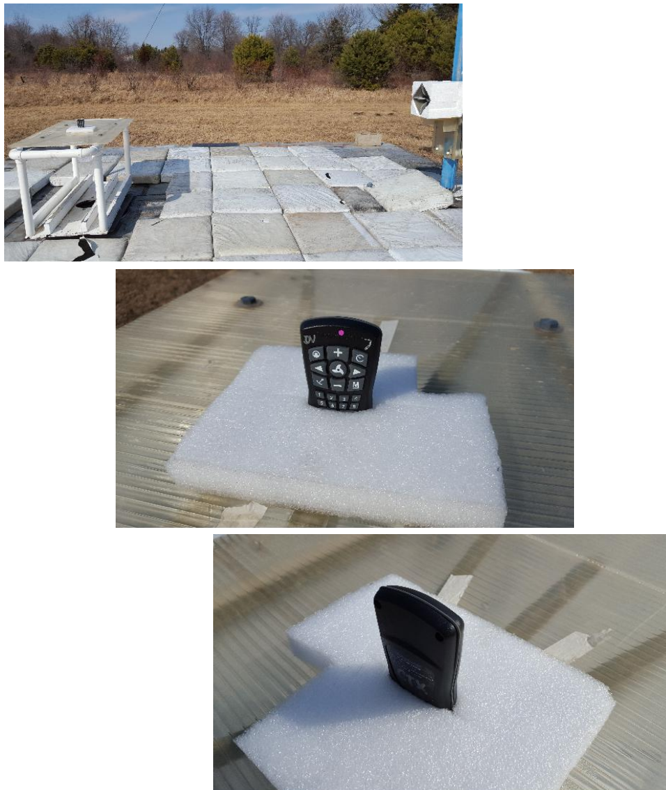
Figure 4: Radiated Emissions Test Setup Photograph(s).
