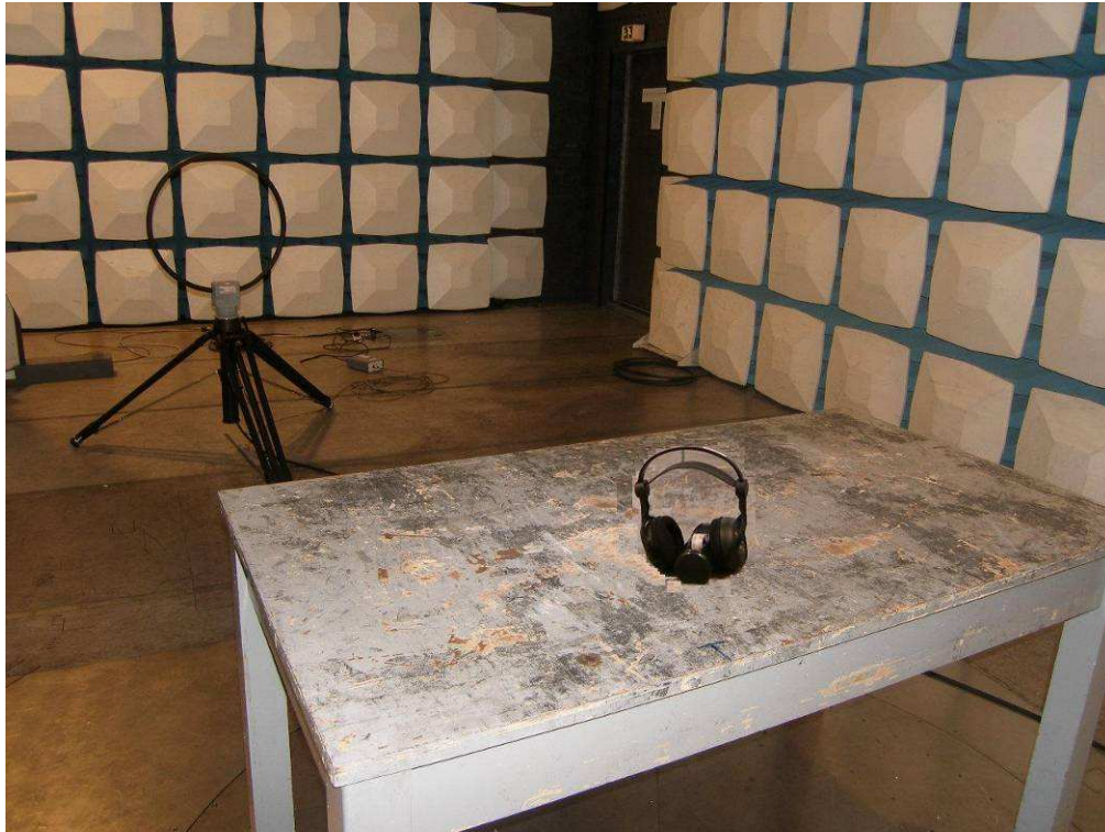
Photograph 2: Set-up for Radiated Emissions (30MHz-1GHz), receiver
