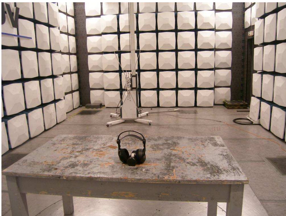
Photograph 2: Set-up for Radiated Emissions (30MHz-1GHz), receiver
