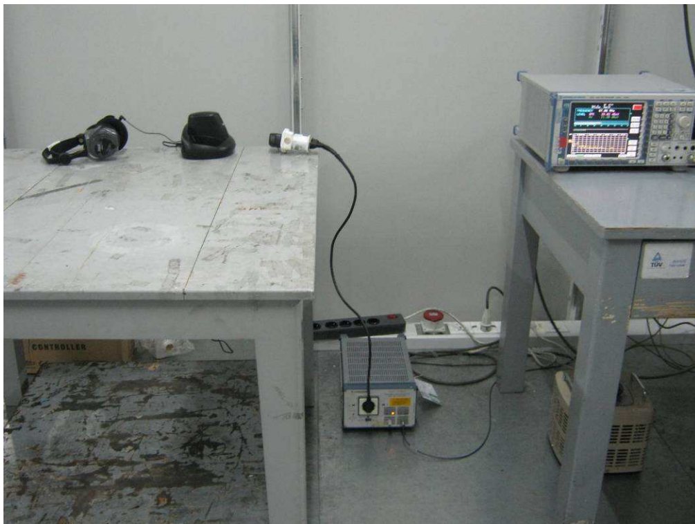
Photograph 4: Set-up for Conducted Emissions
