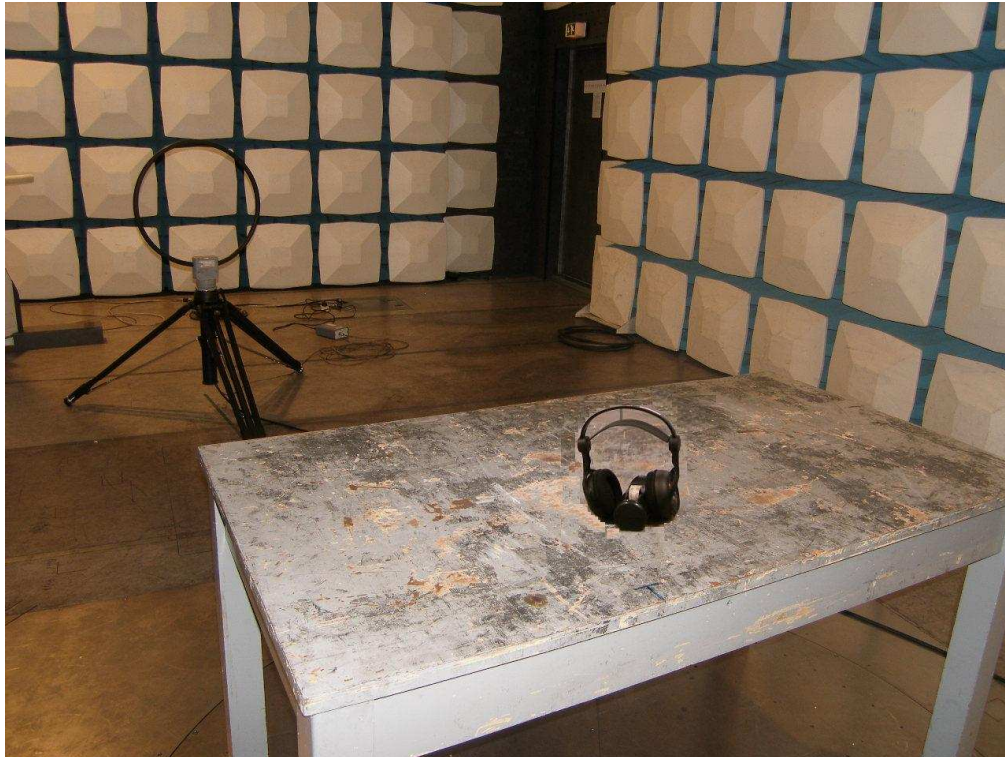
Photograph 2: Set-up for Radiated Emissions (30MHz-1GHz), receiver
