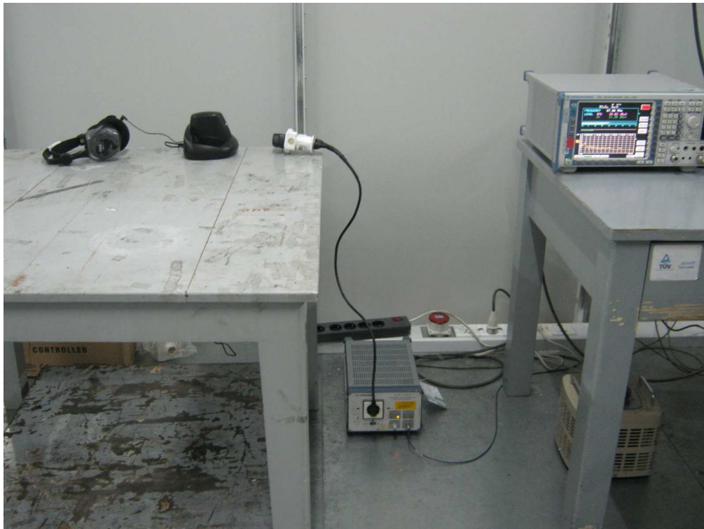
Photograph 4: Set-up for Conducted Emissions
