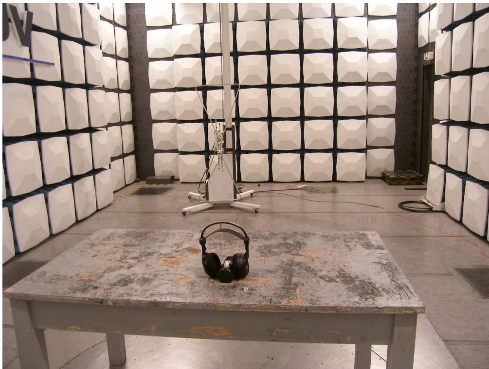
Photograph 2: Set-up for Radiated Emissions (30MHz-1GHz), receiver
