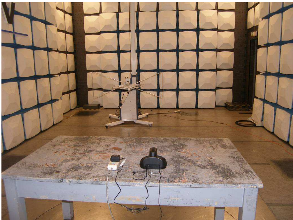
Photograph 2: Set-up for Radiated Emissions (30MHz-1GHz), transmitter
