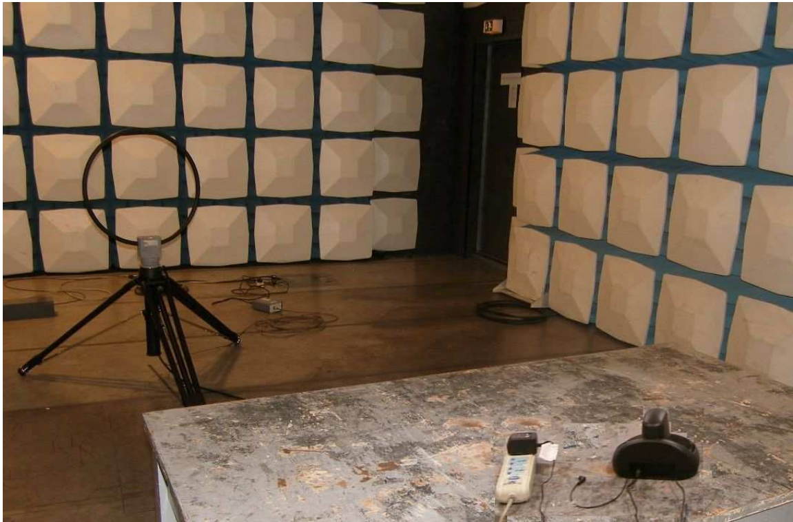
Photograph 2: Set-up for Radiated Emissions (30MHz-1GHz), transmitter
