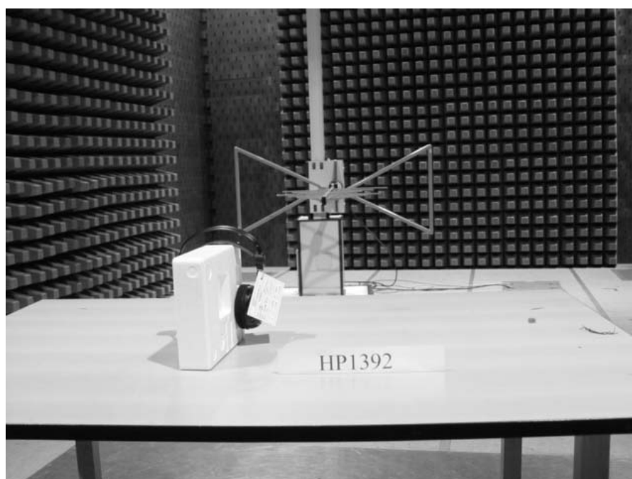
Photograph 2: Set-up for Radiation Measurement Below 1GHz
