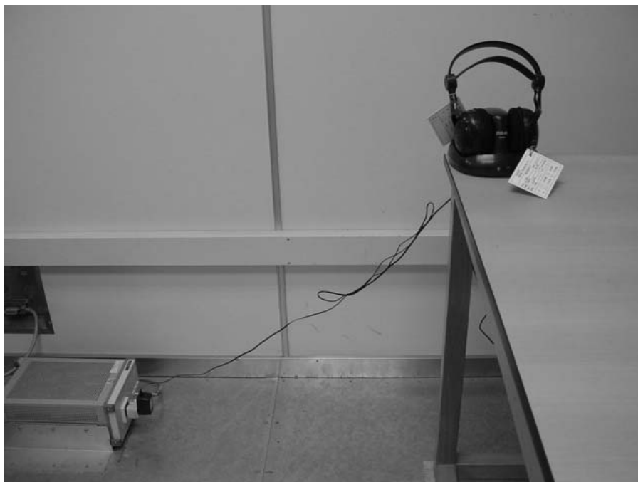
Photograph 1: Set up for Conducted Emission on AC Mains of AC/DC adaptor of HP1391
