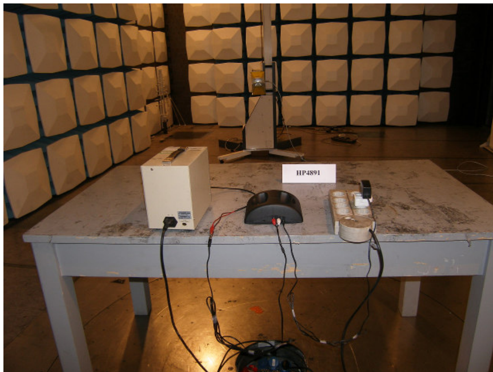
Photograph 3: Set-up for Radiation Measurement Above 1GHz
