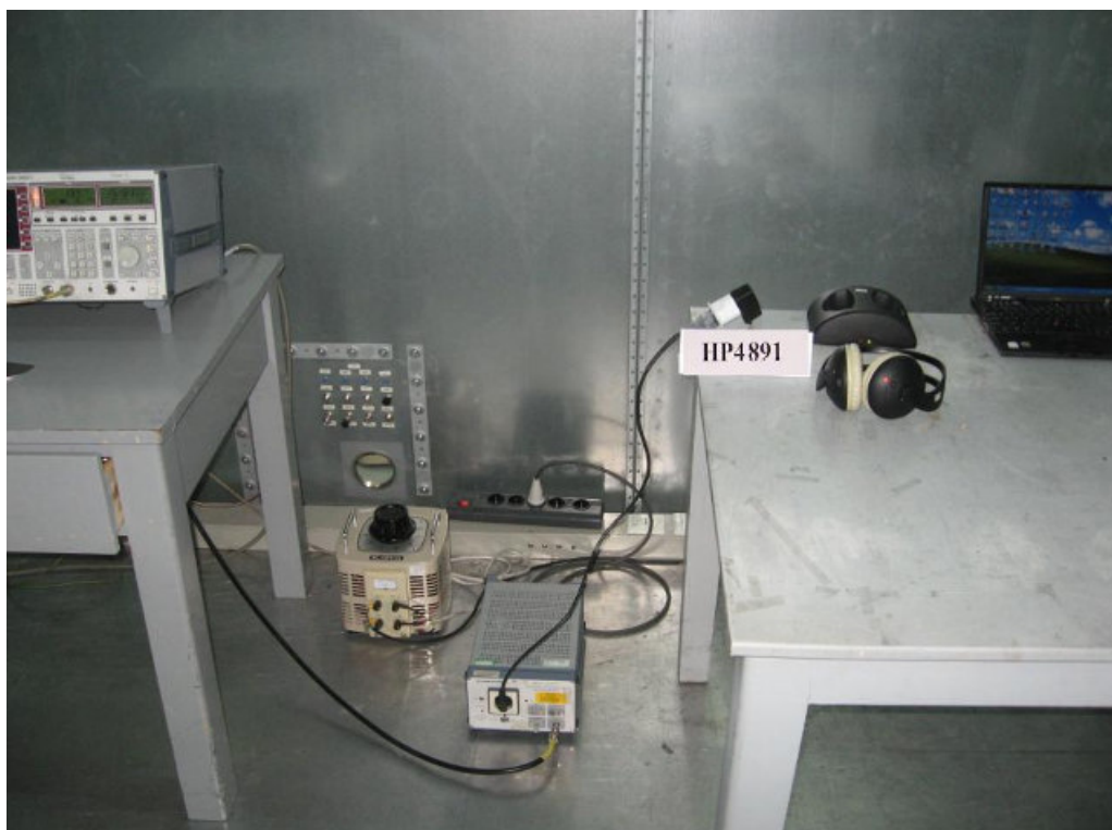
Photograph 1: Set-up for Conducted Emission on AC Mains
