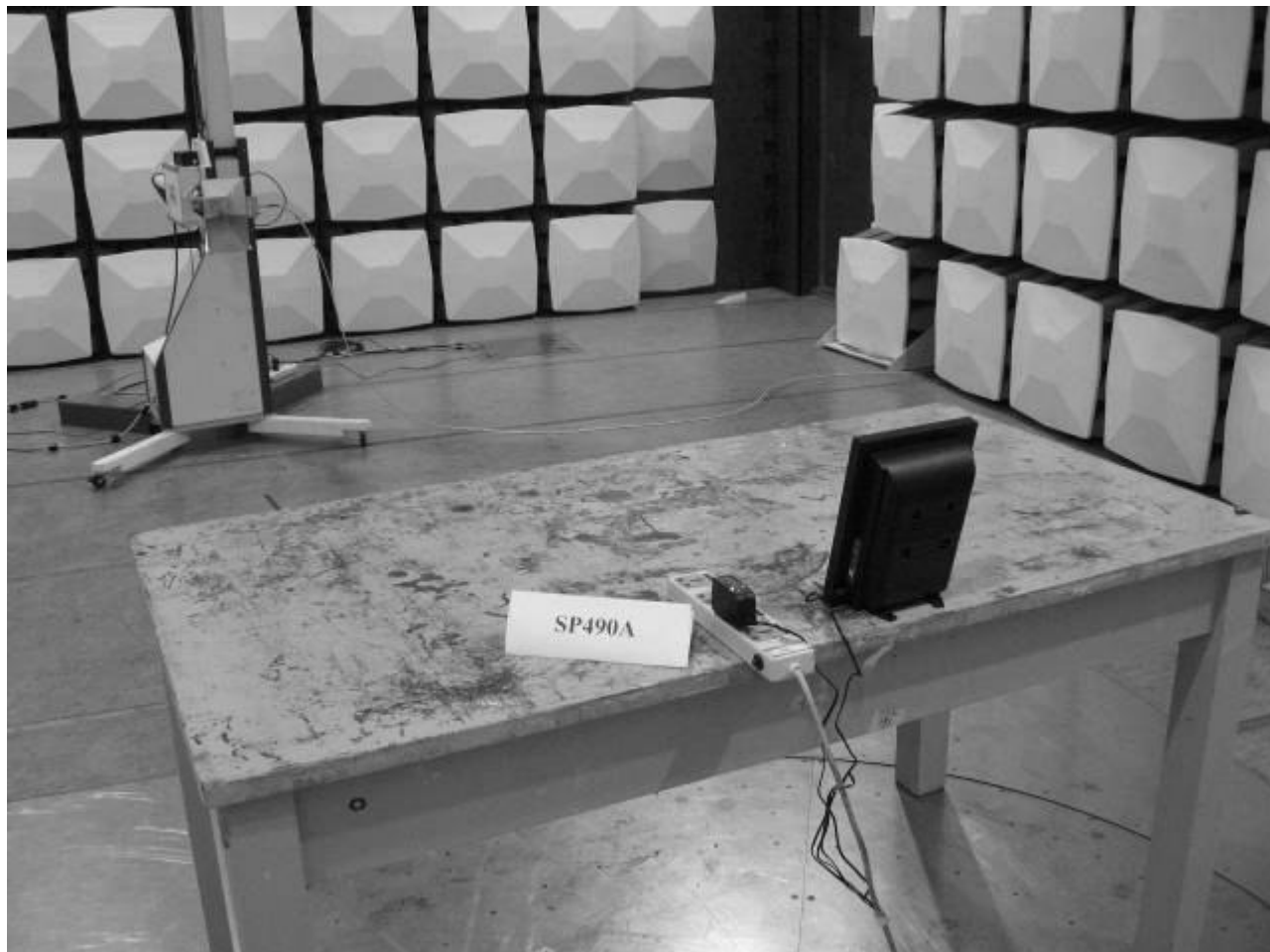
Photograph 3: Set-up for Radiation Measurement Above 1GHz
