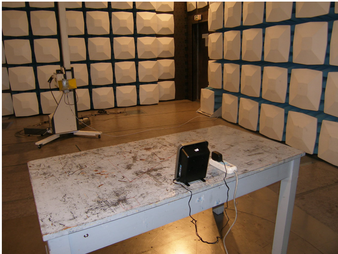
Photograph 3: Set-up for Radiation Measurement Above 1GHz
