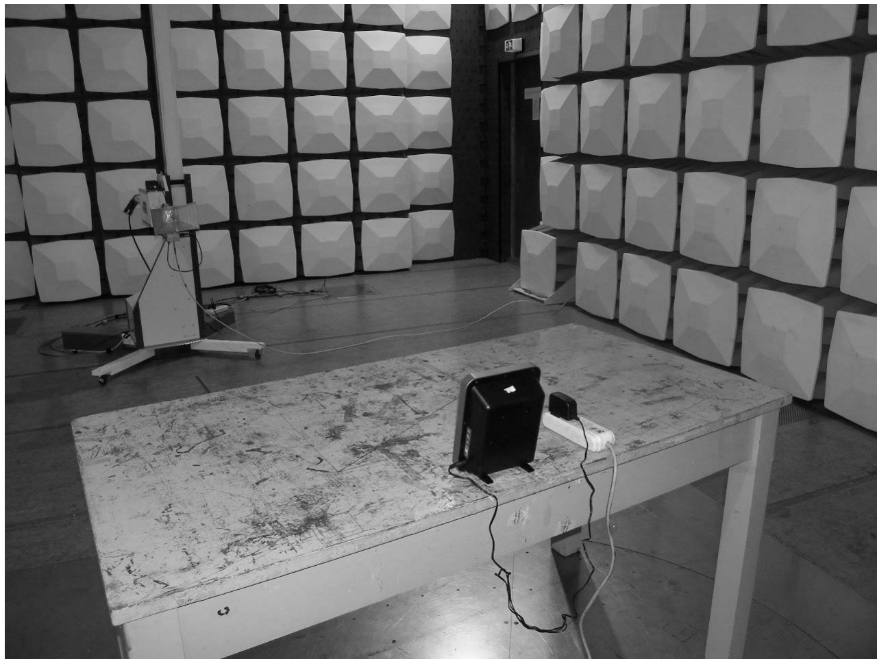
Photograph 3: Set-up for Radiation Measurement Above 1GHz
