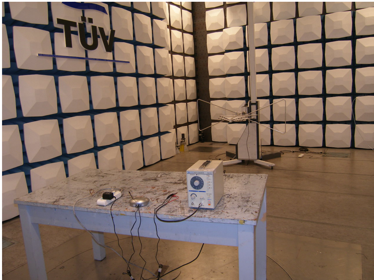
Photograph 2: Set-up for Radiation Measurement Below 1GHz
