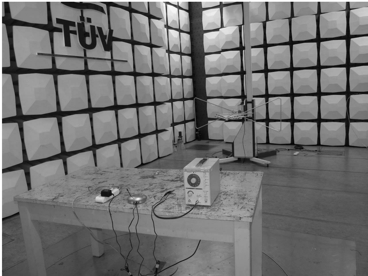
Photograph 2: Set-up for Radiation Measurement Below 1GHz
