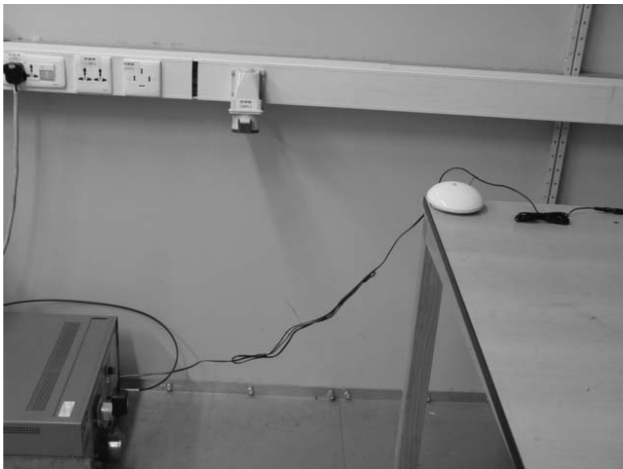
Photograph 1: Set-up for Conducted Emission on AC Mains
