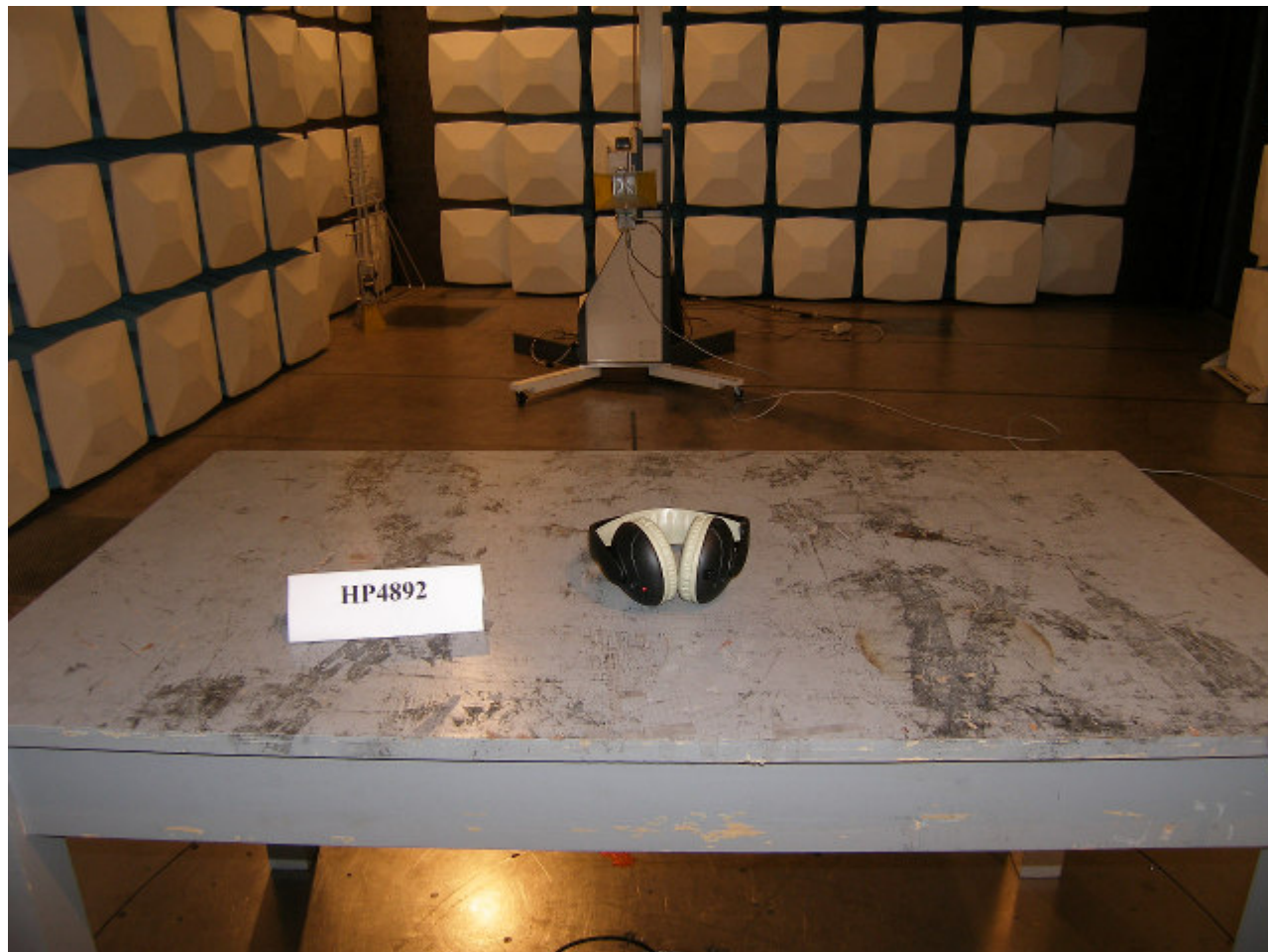
Photograph 2: Set-up for Radiation Measurement above 1GHz
