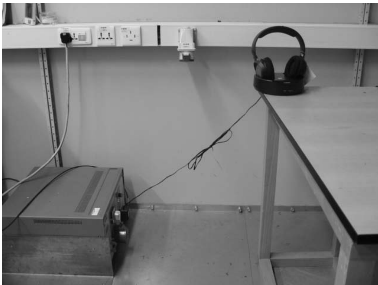
Photograph 1: Set-up for Conducted Emission on AC Mains
