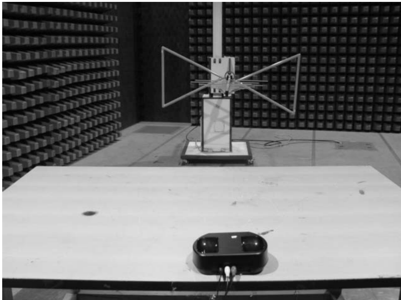
Photograph 2: Set-up for Radiation Measurement Below 1GHz
