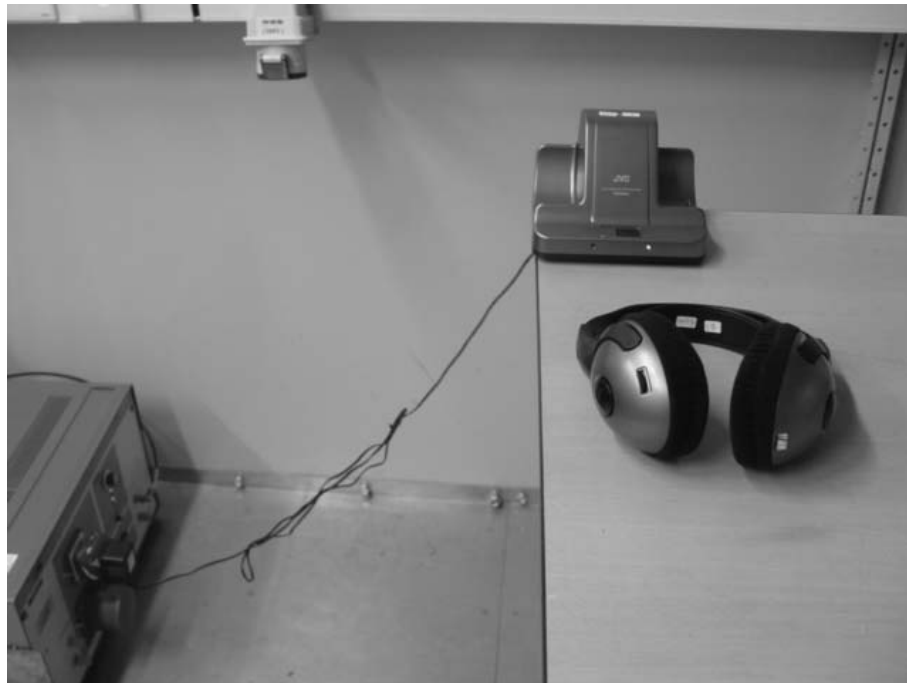
Photograph 1: Set-up for Conducted Emission on AC Mains
