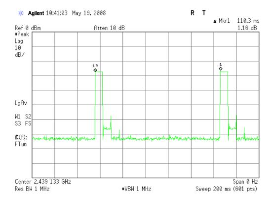
The average time of occupancy in the specified 6 second period (15 channel \*0.4s) is equal to 6\*(# of pulse in 4s/4)\* pulse width.
