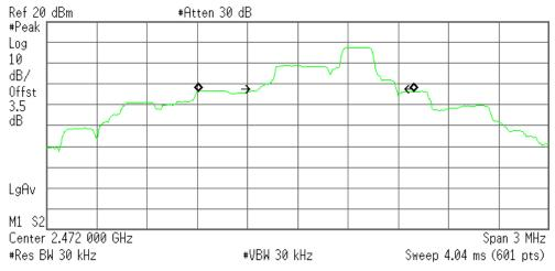
Occupied Bandwidth 1.2876 MHz Occ BW % Pwr **x dB** -20.00 dB
