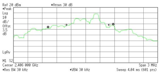
Occupied Bandwidth 1.3534 MHz Occ BW % Pwr 99.00 % **x dB** -20.00 dB
