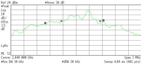
Occupied Bandwidth 1.3432 MHz Occ BW % Pwr 99.00 % **x dB** -20.00 dB
