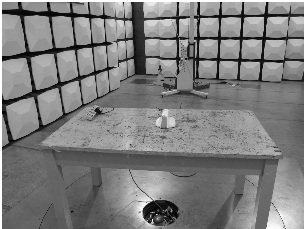
Photograph 3: Set-up for Radiation Measurement above 1GHz
