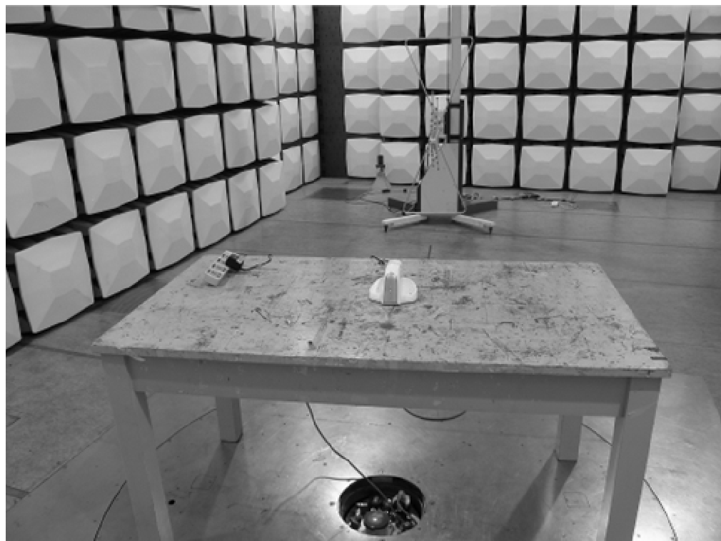
Photograph 3: Set-up for Radiation Measurement above 1GHz
