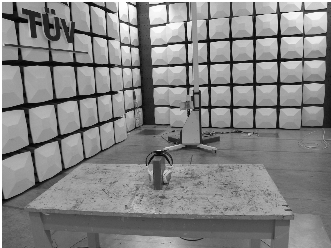
Photograph 2: Set-up for Radiation Measurement above 1GHz
