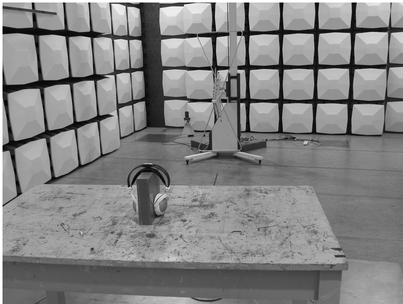
Photograph 1: Set-up for Radiation Measurement below 1GHz
