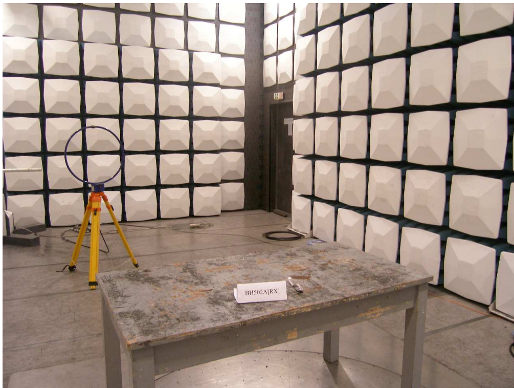
Photograph 4: Set-up for Spurious Emissions (9kHz-30MHz)
