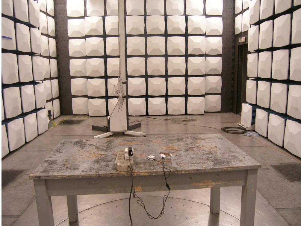
Photograph 2: Set-up for Radiated Emissions, above 1GHz
