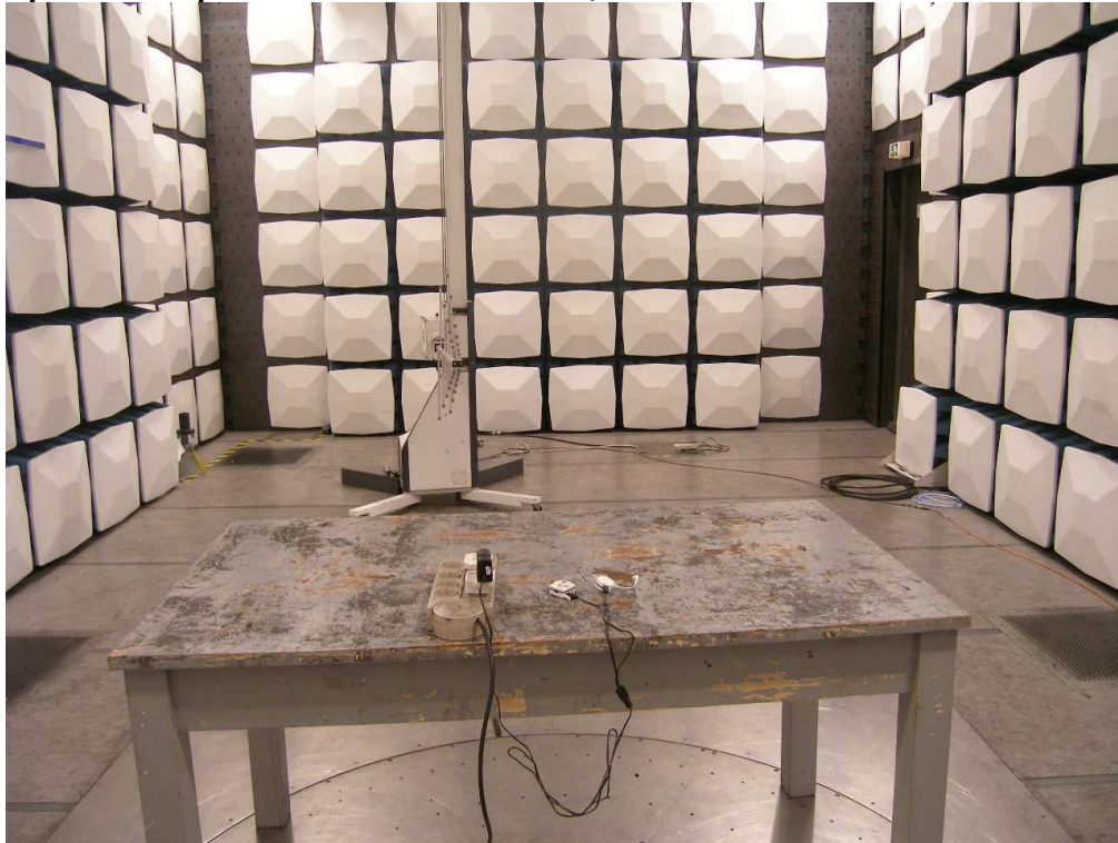
Photograph 2: Set-up for Radiated Emissions, above 1GHz
