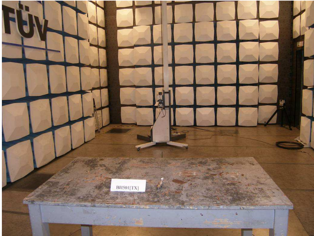
Photograph 7: Set-up for Spurious Emissions (18GHz-26GHz)
