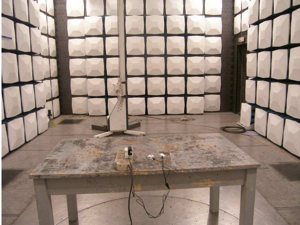
Photograph 2: Set-up for Radiated Emissions, above 1GHz
