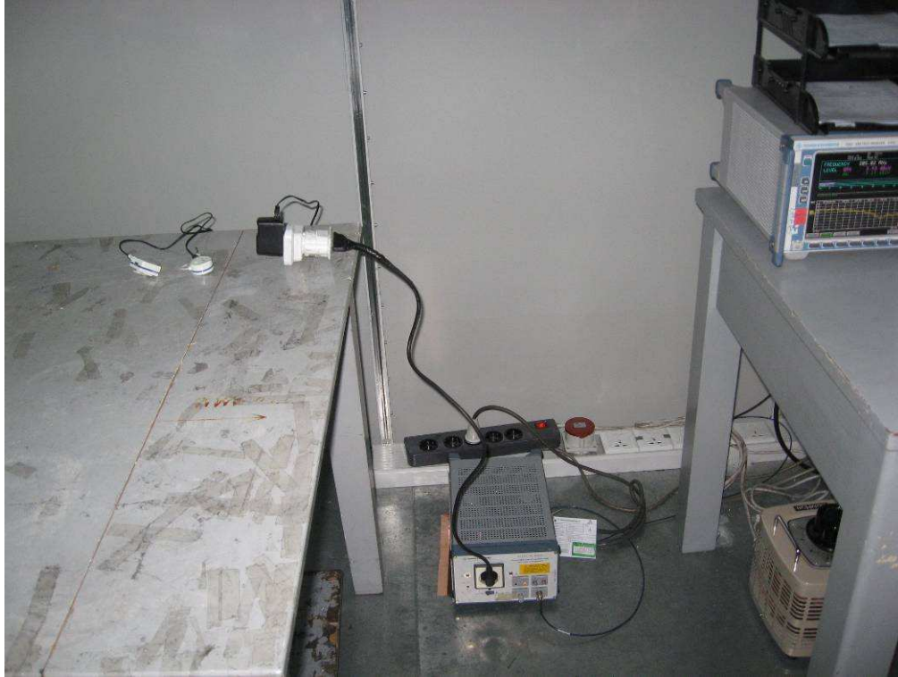
Photograph 4: Set-up for Spurious Emissions (9kHz-30MHz)
