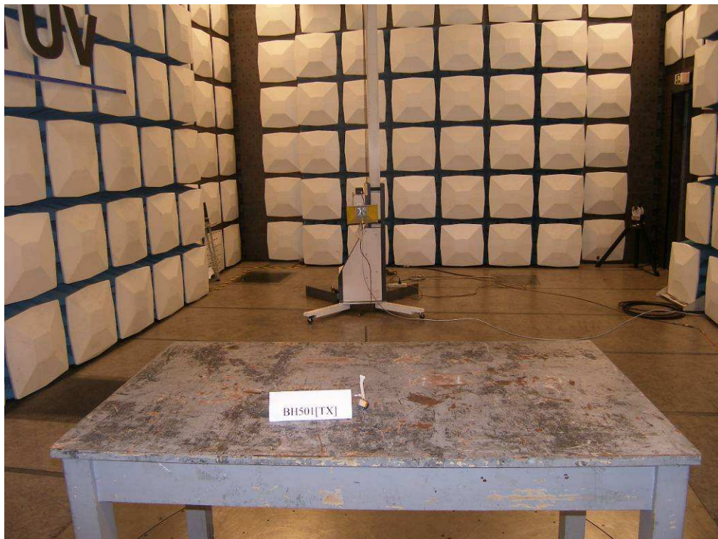
Photograph 6: Set-up for Spurious Emissions (1GHz-18GHz)
