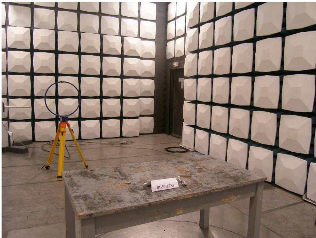
Photograph 4: Set-up for Spurious Emissions (9kHz-30MHz)
