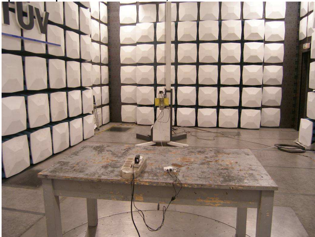
Photograph 2: Set-up for Radiated Emissions, above 1GHz
