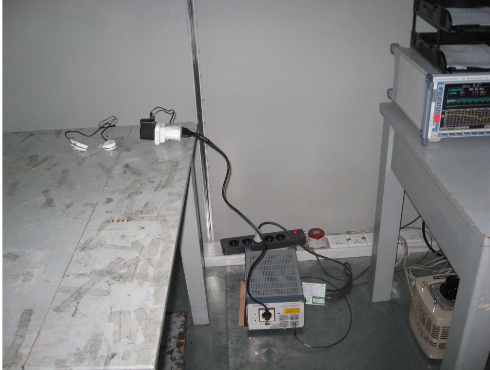
Photograph 4: Set-up for Spurious Emissions (9kHz-30MHz)
