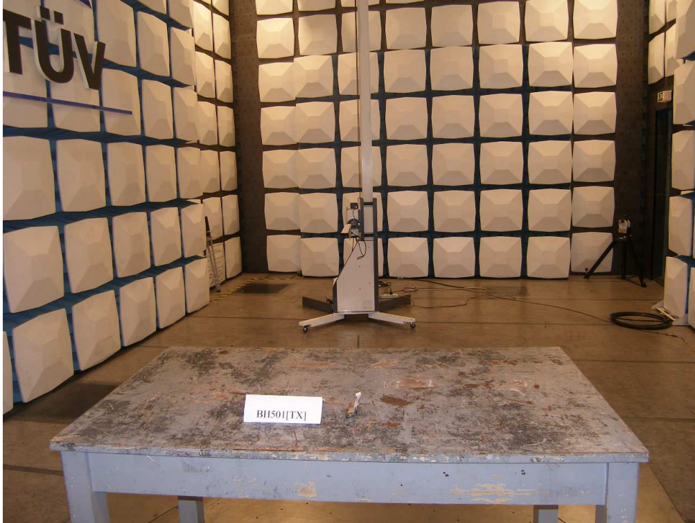
Photograph 7: Set-up for Spurious Emissions (18GHz-26GHz)
