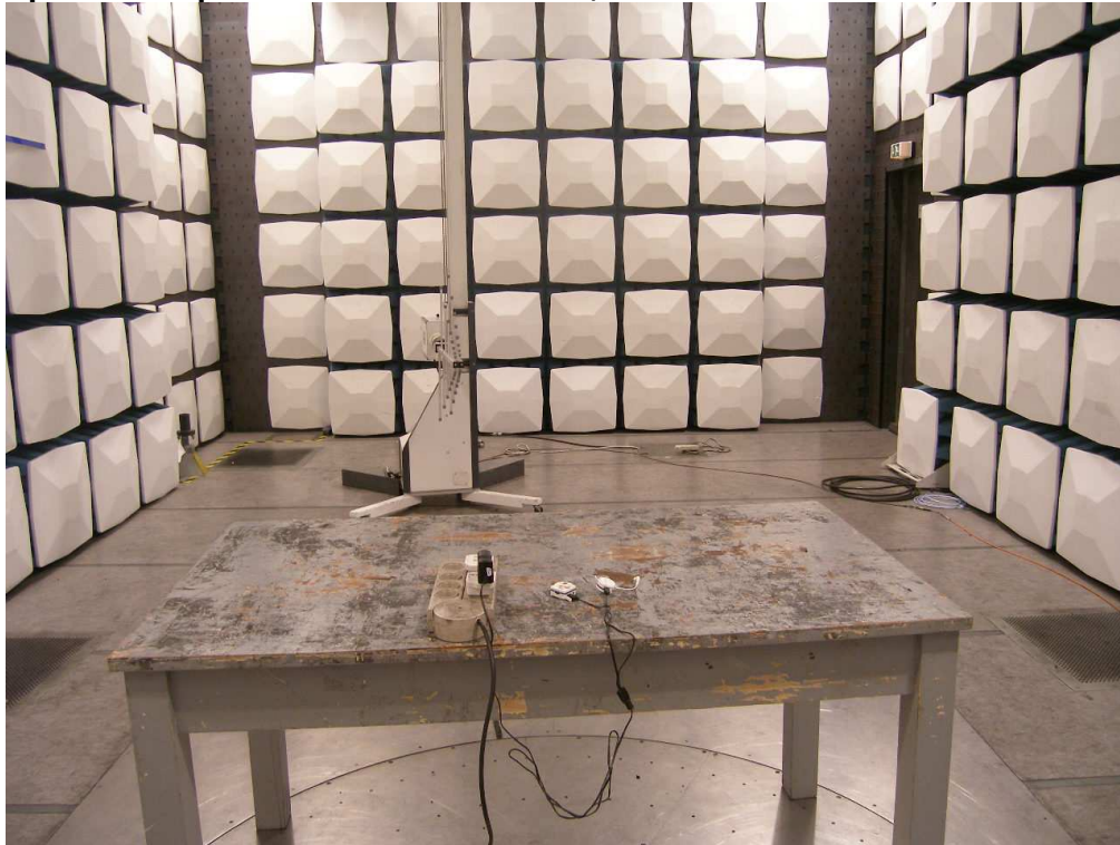
Photograph 2: Set-up for Radiated Emissions, above 1GHz
