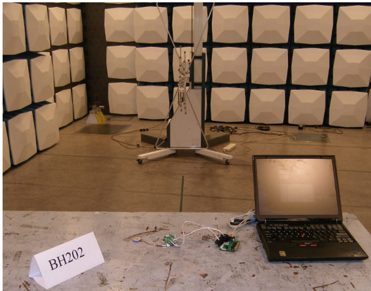
Photograph 2: Set-up for Radiation Measurement below 1GHz
