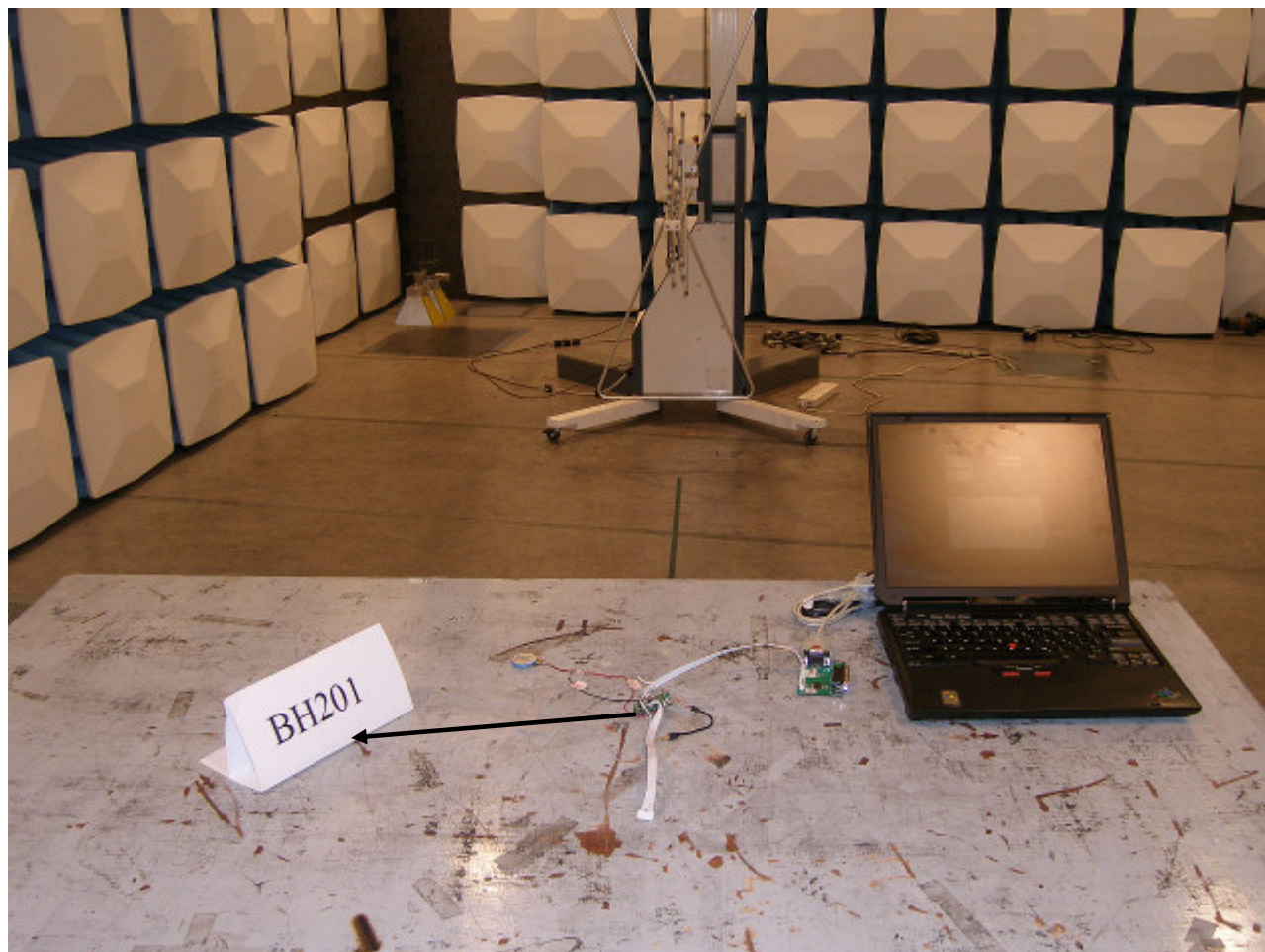
Photograph 2: Set-up for Radiation Measurement below 1GHz
