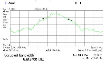
Transmit Freq Error -17.978 kHz x dB Bandwidth 887.593 kHz
