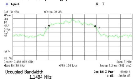
Transmit Freq Error -8.573 kHz x dB Bandwidth 1.210 MHz
