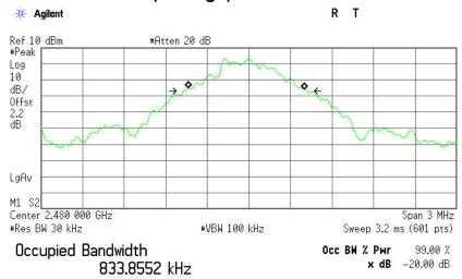
Transmit Freq Error -17.437 kHz x dB Bandwidth 889.042 kHz
