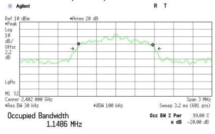
Transmit Freq Error 1.618 kHz x dB Bandwidth 1.208 MHz
