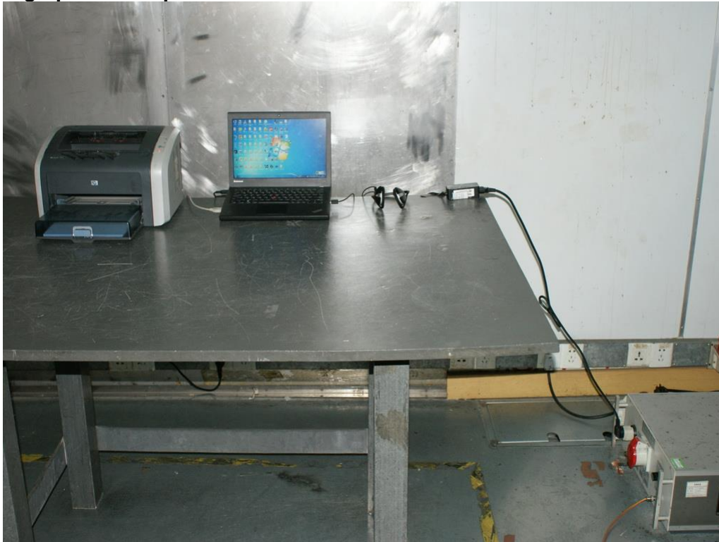
Photograph 2: Set-up for Spurious Emissions for below 30MHz
