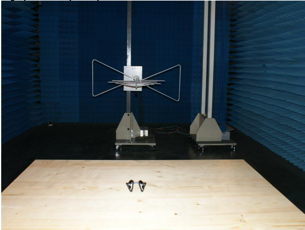
Photograph 4: Set-up for Spurious Emissions for 1 - 18GHz
