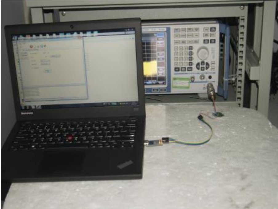
Photograph 2: Set-up for Radiated Spurious Emission (9kHz ~ 30MHz)
