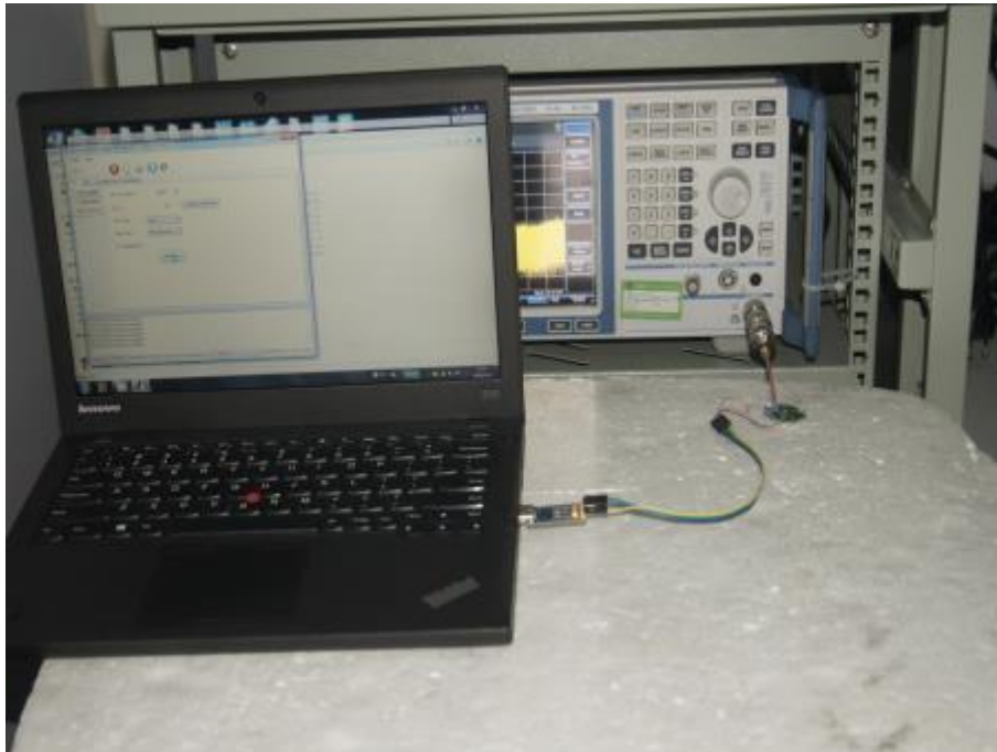
Photograph 2: Set-up for Radiated Spurious Emission (9kHz ~ 30MHz)
