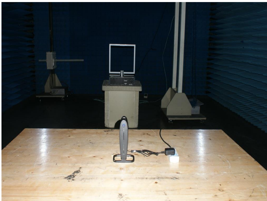
Photograph 4: Set-up for Radiated Spurious Emission, 9KHz - 30MHz
