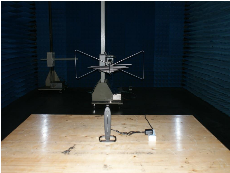
Photograph 5: Set-up for Radiated Spurious Emission, 30MHz - 1GHz
