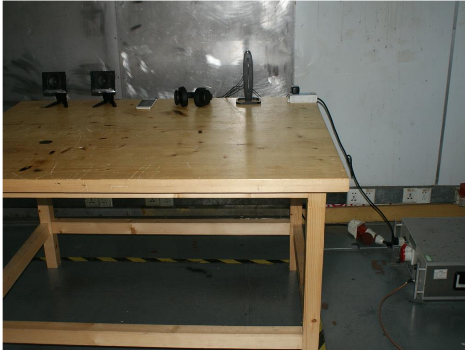
Photograph 1: Set-up for Conducted Emission on AC Mains
