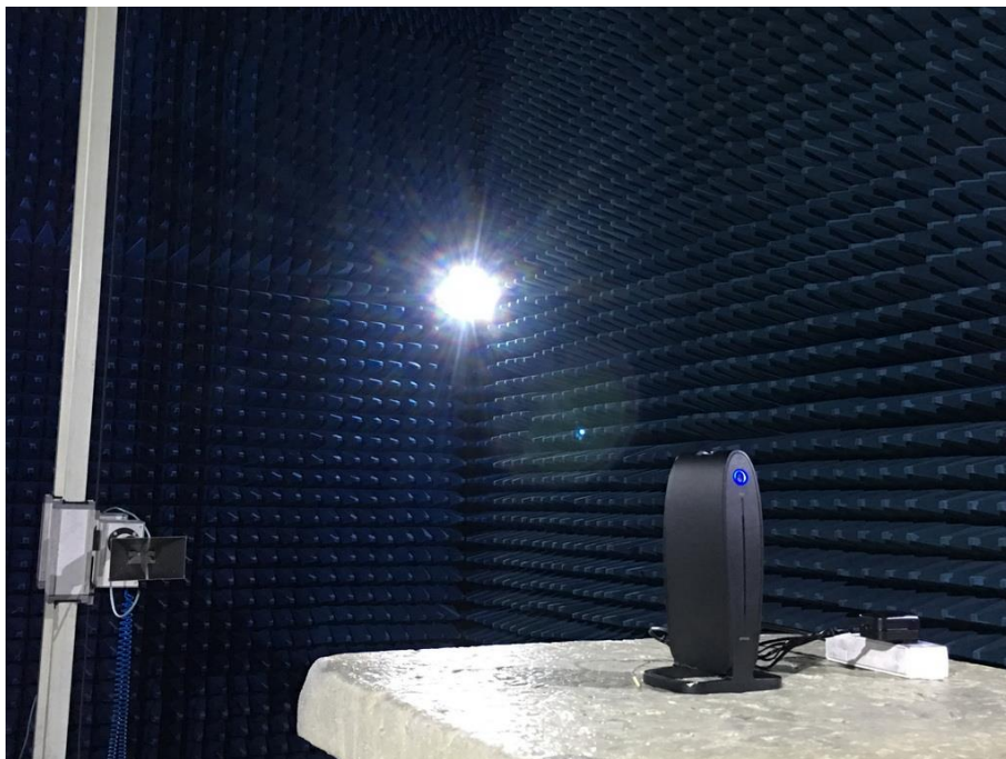
Photograph 6: Set-up for Radiated Spurious Emission, 1GHz - 18GHz
