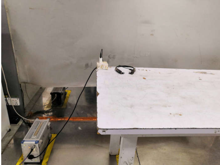
Conducted Emissions Test Setup
