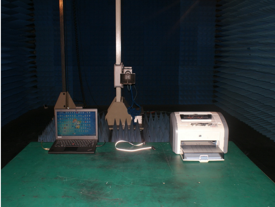
Photograph 7: Set-up for Radiated Emissions, above 1GHz
