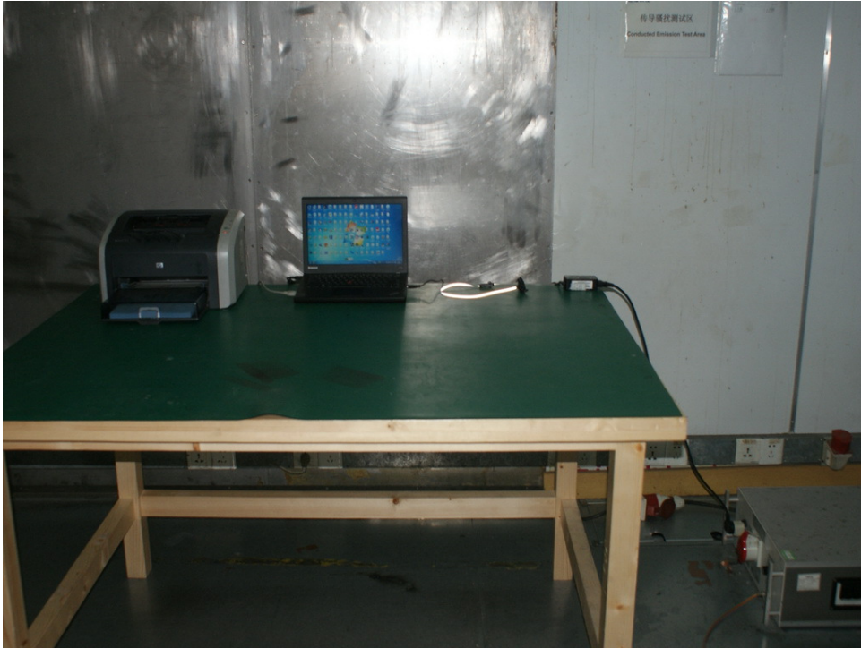
Photograph 6: Set-up for Radiated Emissions, below 1GHz
