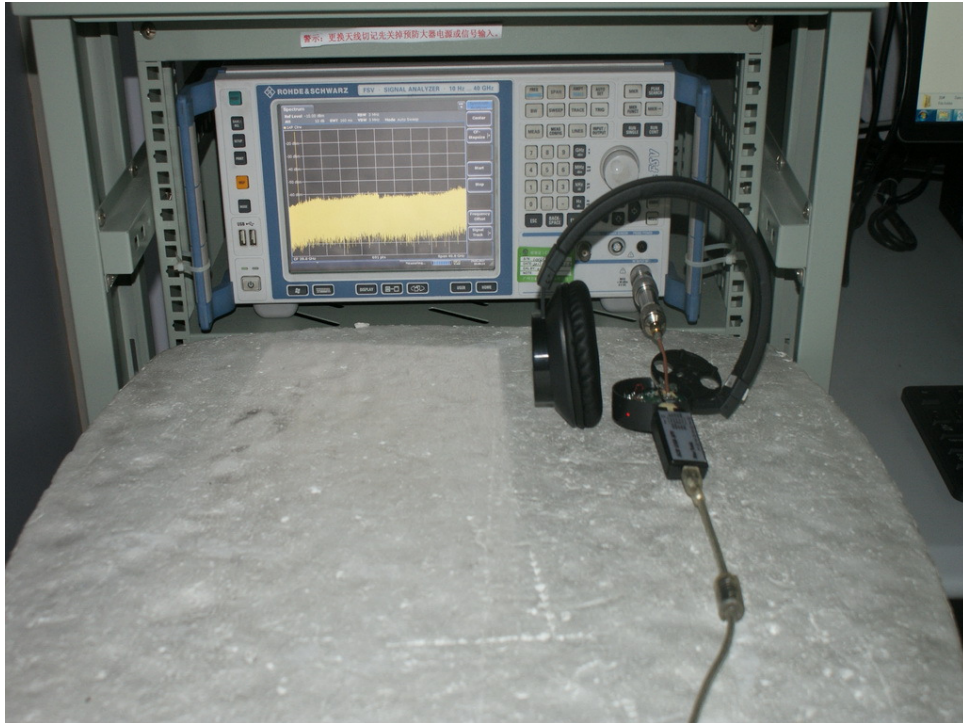
Photograph 2: Set-up for Spurious Emissions (9kHz-30MHz)
