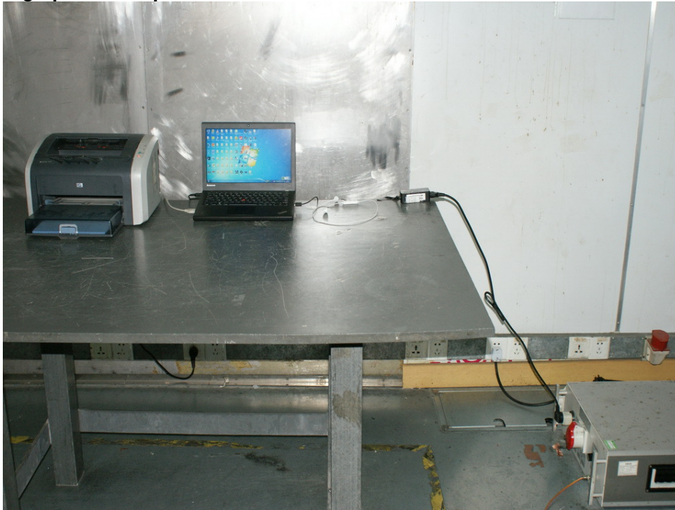
Photograph 6: Set-up for Radiated Emissions below 1GHz
