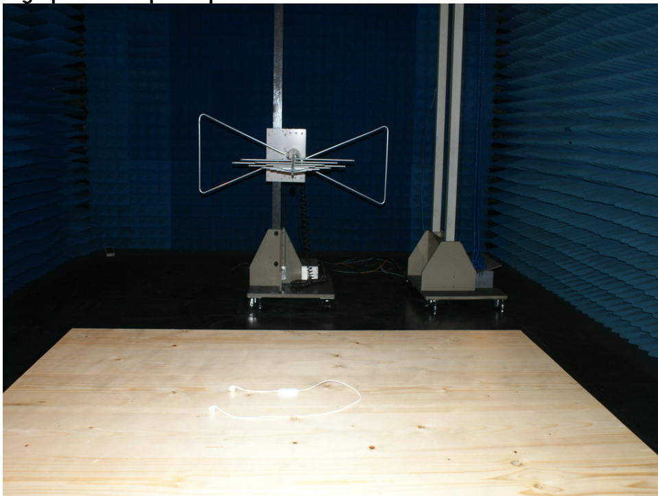
Photograph 2: Set-up for Spurious Emissions for 30 - 1000MHz
