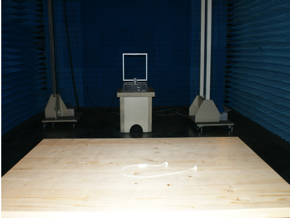
Photograph 2: Set-up for Spurious Emissions for 30 - 1000MHz
