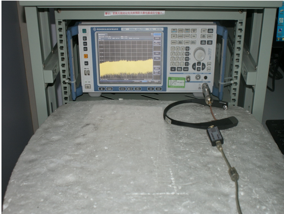
Photograph 2: Set-up for Spurious Emissions (9kHz-30MHz)
