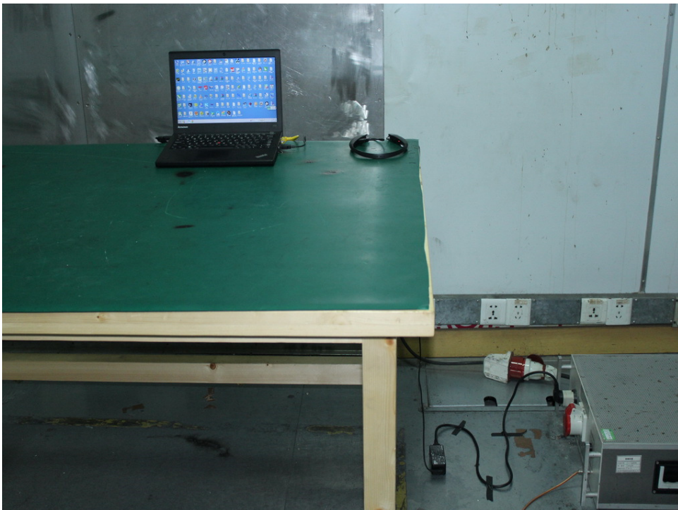
Photograph 6: Set-up for Conducted Emissions
