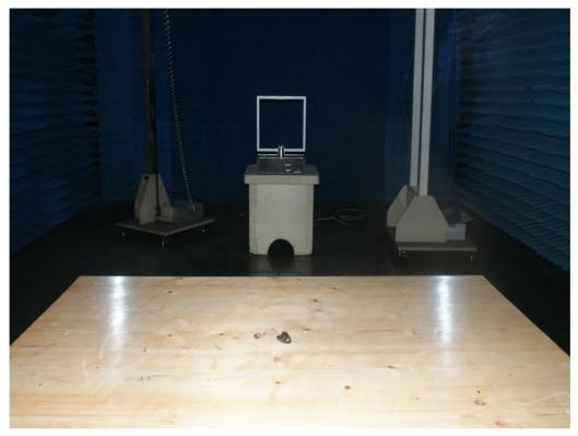
Photograph 2: Set-up for Spurious Emissions (30MHz-1GHz)
