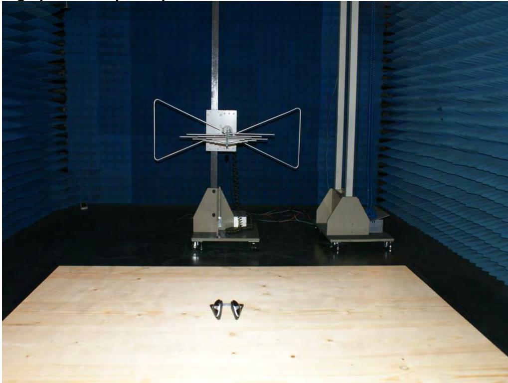
Photograph 4: Set-up for Spurious Emissions for 1 - 18GHz
