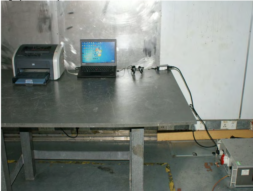
Photograph 2: Set-up for Spurious Emissions for below 30MHz
