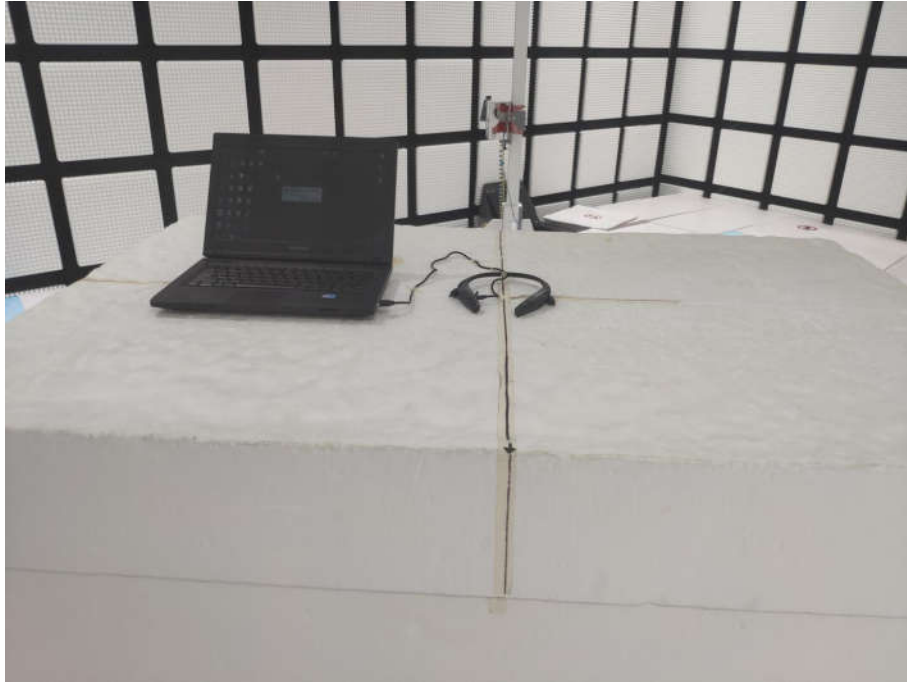
Radiated spurious emission Test Setup-3(Above 1GHz)
