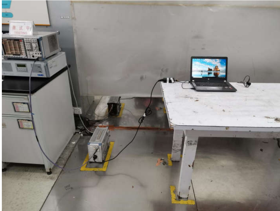
AC Conducted Emissions Test Setup
