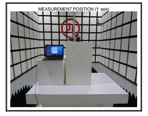
RADIATED RF MEASUREMENT SETUP (ABOVE 1 GHz)
