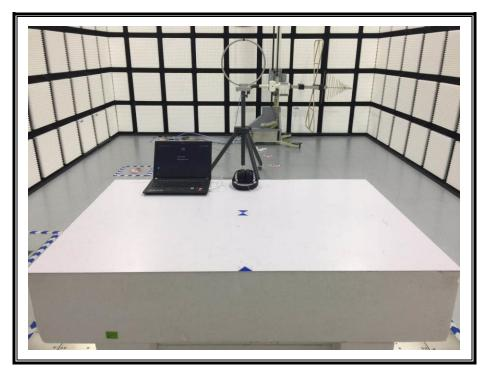
POWERLINE CONDUCTED EMISSIONS MEASUREMENT SETUP
